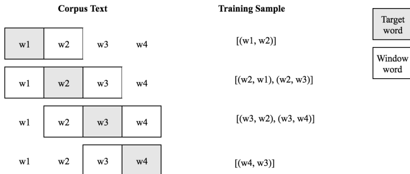
Figure 7: Skip-gram representations of training samples (at each training iteration) with a window size = 1
